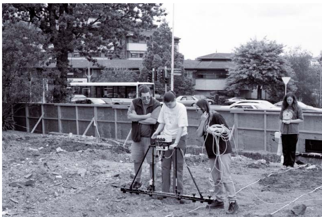
Figure 19. Resistivity meter RM15 in front of the fluxgate magnetometer FM9
