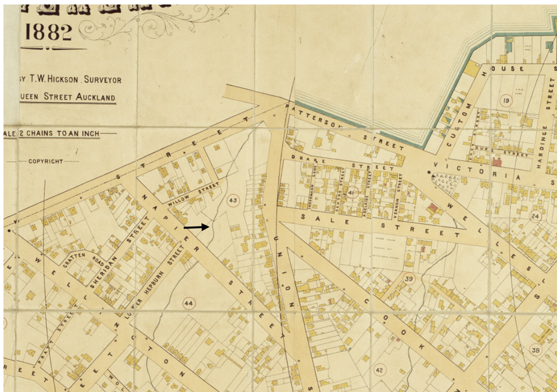
Figure 12. Hickson's 1882 map of Auckland (detail), showing the area from Patteson Street to Wellington Street, and the line of the stream/culvert (arrow). The Drake Street to Patteson Street reclamation is shown to be completed, with a sea wall in place. (Sir George Grey Special Collections, Auckland Libraries, NZ Maps 91)
