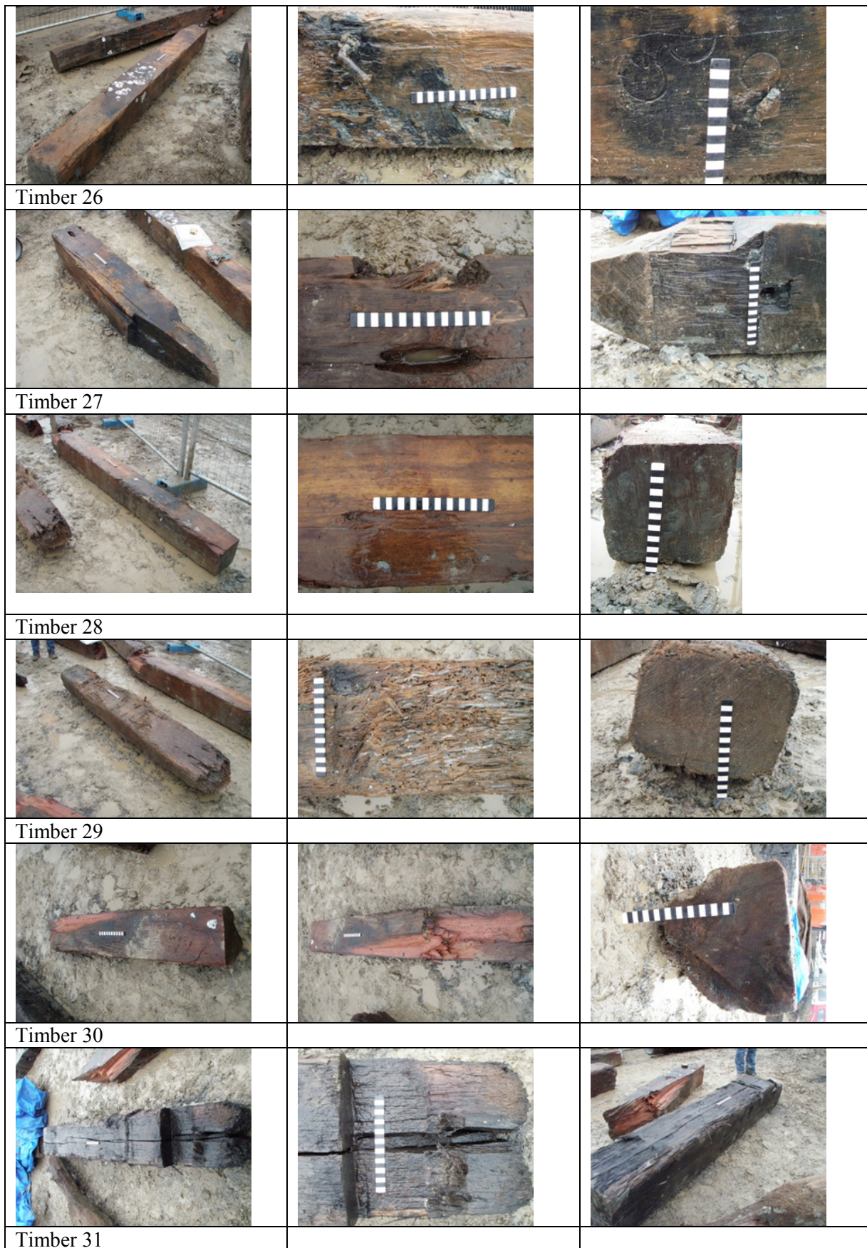
Figure 92. Selected photographs of the 11 timber piles recovered during the tunnel excavations
