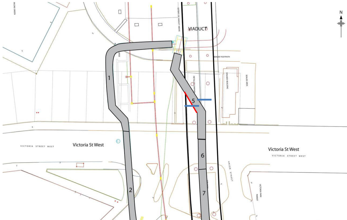
Figure 60. Location of the two timber walls within the Area 5 trench : the red line indicates the location of the section drawing, the blue lines indicate the orientation of the two walls
