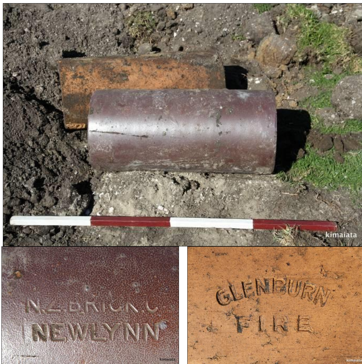
Figure 62. Drainage field tiles: N.Z. BRICK CO NEWLYNN (L), and GLENBURN FIRE (R)
