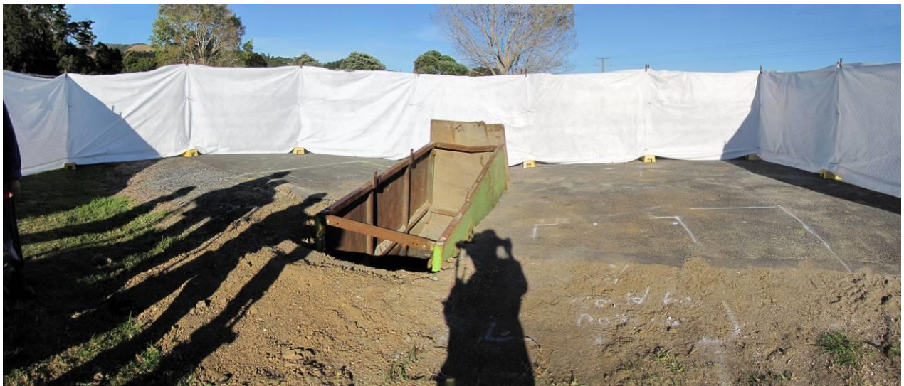
Figure 23. Areas of interest identified by GPR marked out in white paint
