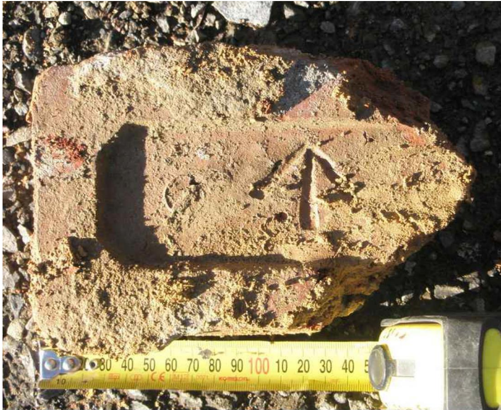
Figure 5.14 Sample of press-moulded prison brick from the stormwater trench in front of the Carillon (scale in cm)
