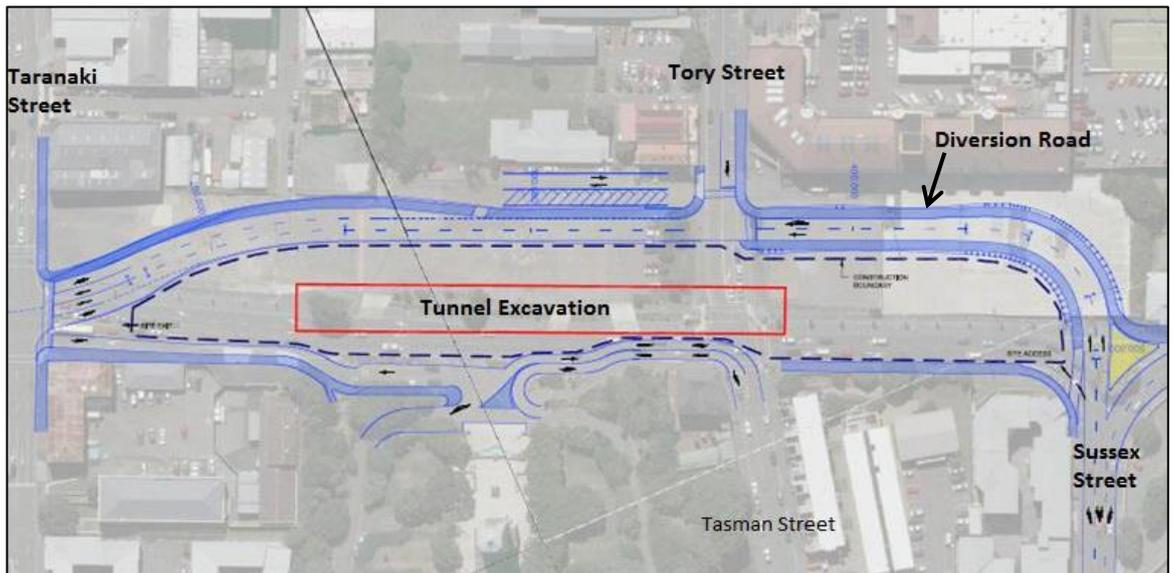
Figure 1.6 The diversion road for SH1 (arrowed) with the red outline defining the tunnel excavation area
