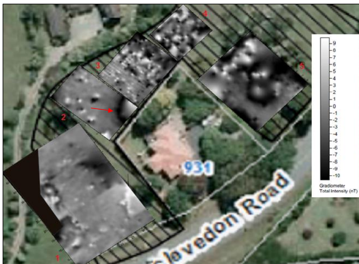
Figure 4.1 Image of the processed magnetic data from magnetometer survey of Ring's Redoubt with the curving anomaly that may indicate the site of the north-western bastion (arrowed). NB. The greyscale measures magnetic intensity with white indicating a strongly magnetic response while black is weak; the numbers demarcate the individual survey blocks
