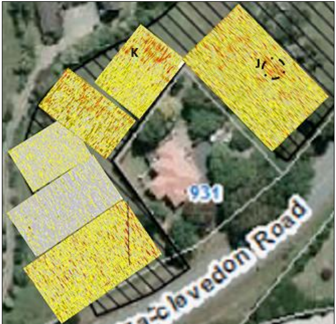
Figure 4.9 GPR time-slice at 0.50m depth illustrating the continued presence of anomaly (K) and with increasing intensity in survey block 5; anomaly J in survey block 6 and the pipeline to the west and southwest of the house in survey block 1 indicated by the line
