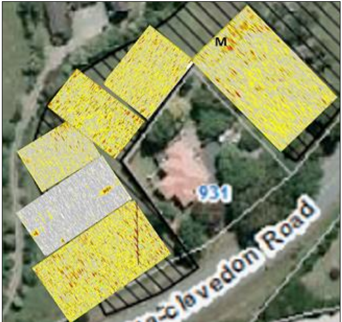
Figure 4.12 GPR time-slice at 1.50m depth illustrating the presence of a linear anomaly (M) in survey block 6 to the north of the remains of the redoubt interior platform which potentially indicates the infilled northern redoubt ditch
