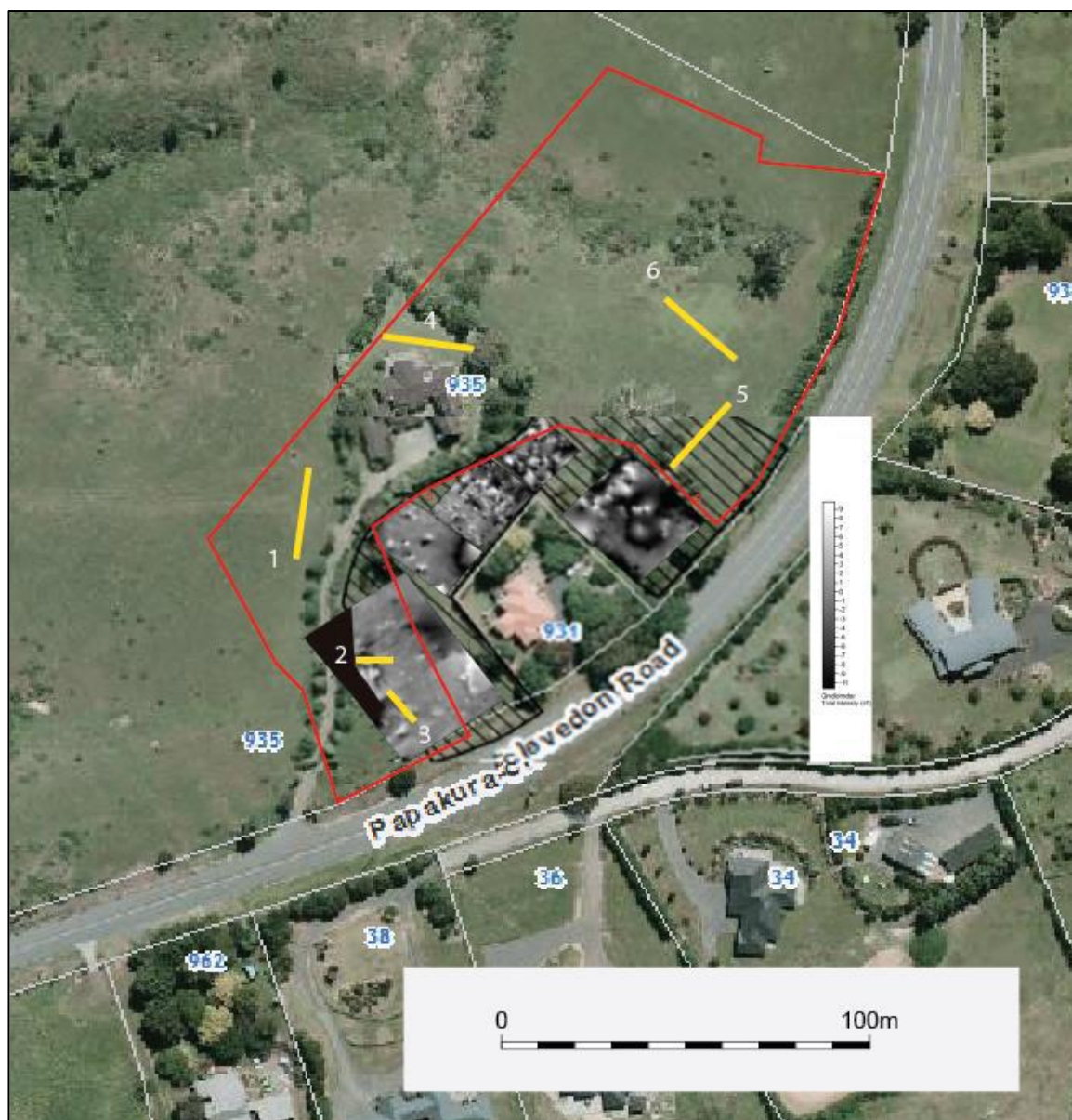
Figure 1.7 Magnetometer survey results and aerial overlay illustrating the location of the six proposed trial trenches excavated for the exploratory investigation. Note that Trench 4 in the back garden of the house at 935 Papakura-Clevedon Road was not excavated as it became clear that the area had been cut and benched over 1.5m at the time the house had been constructed
