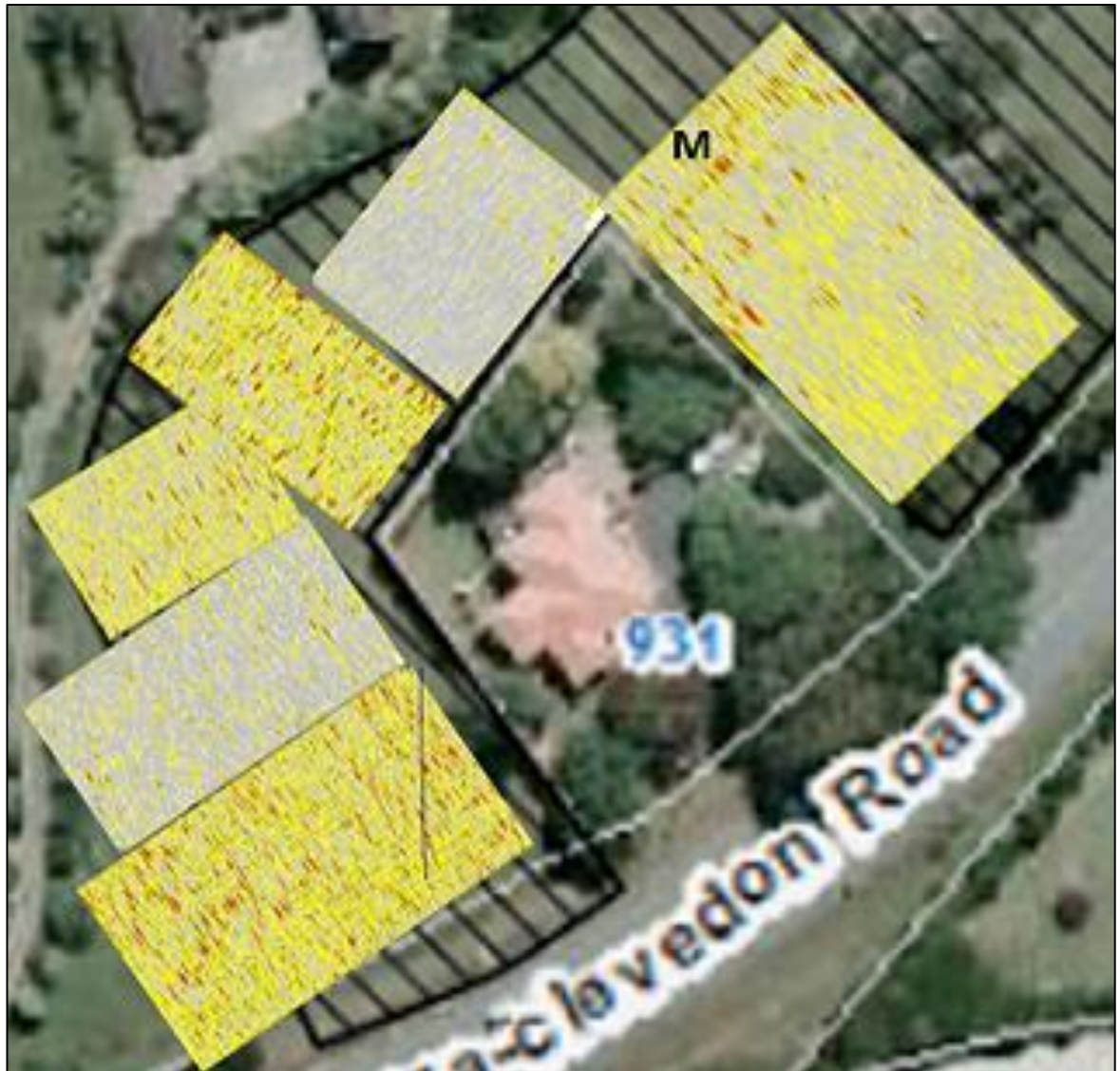
Figure 4.13 GPR time-slice at 2.00m depth demonstrating the linear anomaly (M) to the north of the remains of the redoubt interior, possibly indicating that the northern redoubt ditch has been infilled
