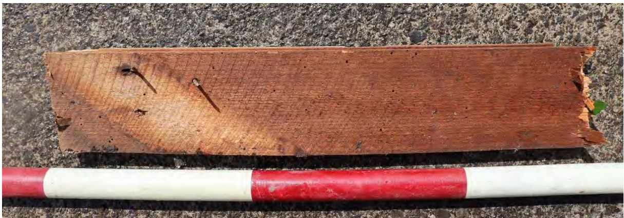
Figure 61. Section of gable plank with circle-sawn cut marks. Scale interval 20cm
