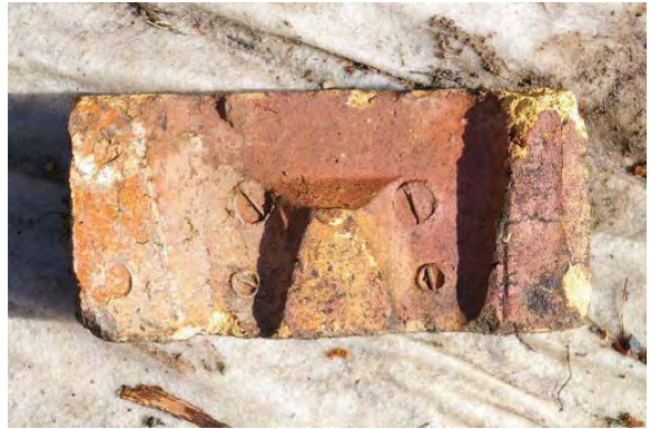
Figure 136. Lower view of chequer brick with mould marks
