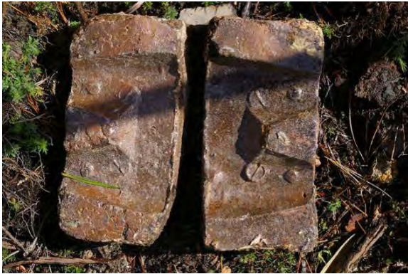
Figure 135. Pair of chequer bricks glazed through use
