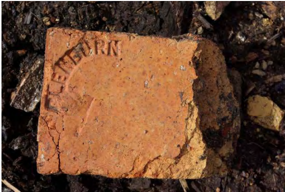
Figure 137. 'GLENBURN' ?firebrick FROM J.J. Craig brickworks, machine pressed
