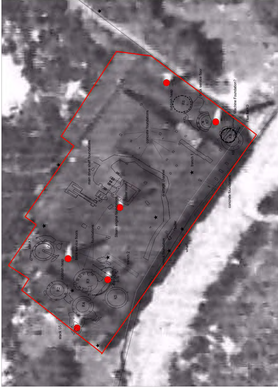
Figure 48. Site features overlaid on 1940s aerial. Note that the aerial is taken at a slightly oblique angle. Approximate locations of stack bases circled in red
