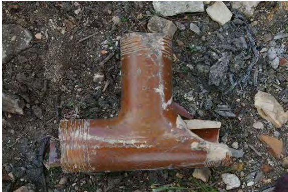
Figure 143. T-junction pipe, possibly pressure pipe, with grooved ends to facilitate junction with other pipes; very thick walled
