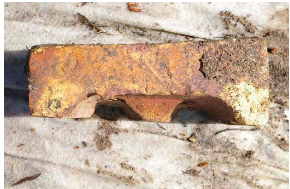
Figure 134. Side view of chequer brick from base of kiln – machine pressed firebrick
