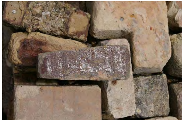
Figure 129. Wire cut partially glazed arch brick
