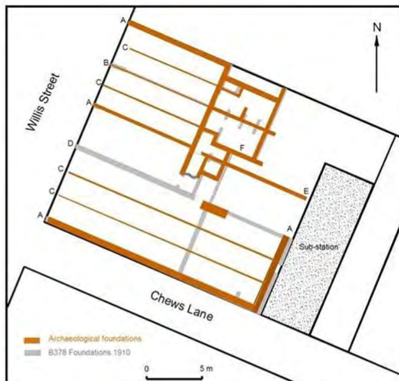
Figure A9.6. Plan showing the archaeological foundations and building footprints fronting Willis Street. A = foundations below external walls, B = foundation below internal wall separating two shops in the same building. C = foundations not beneath walls, probably used to support floor joists. D = foundation below external wall present in the section along the Willis Street road frontage, showing signs of later strengthening. E = a foundation for the external wall of a building erected after 1910. F = external wall of 1910 building annex
