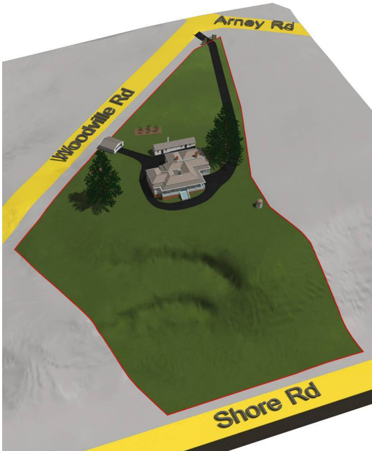
Figure 51. 3D Computer based model using LIDAR data showing reconstructed terraces
