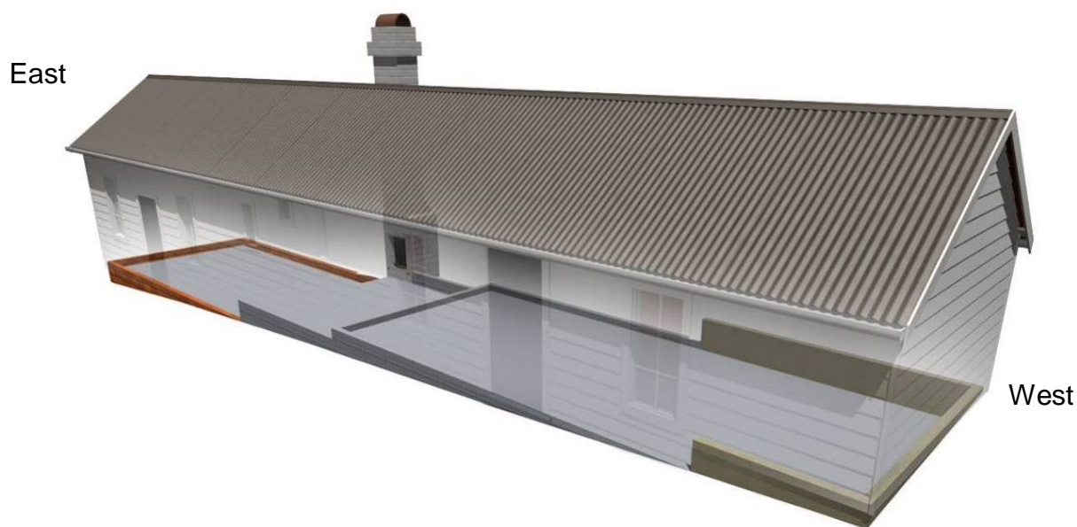
Figure 69. X-Ray view of cottage above showing original floor levels
