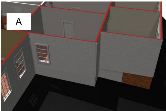
Figure 18. Middle phase of the property with cottage and stables pre-1950s (roofs removed to show interior)
