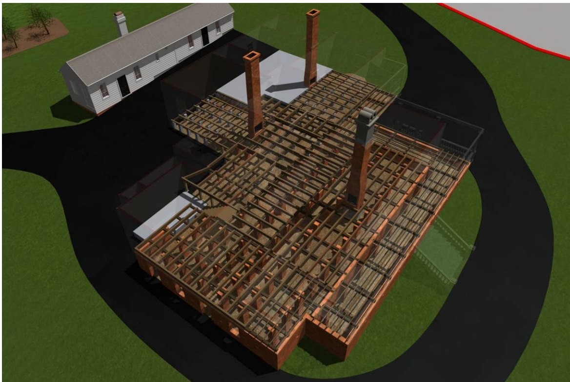
Figure 12. View through the house showing floor joists and foundations
