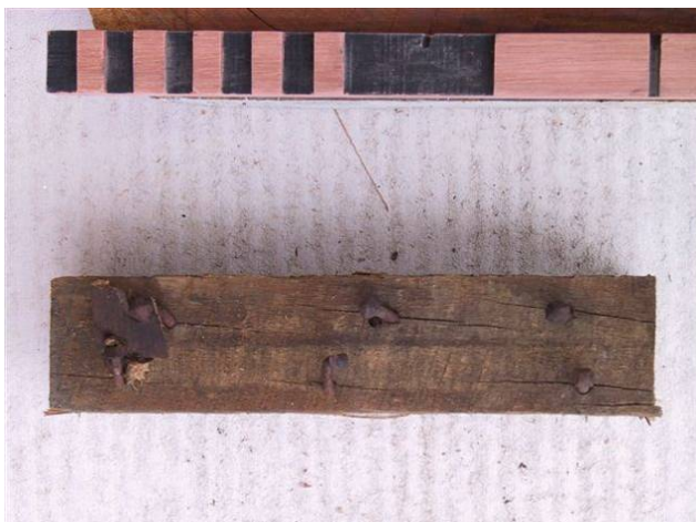
Figure 45. Bearer for wall panelling in cottage
