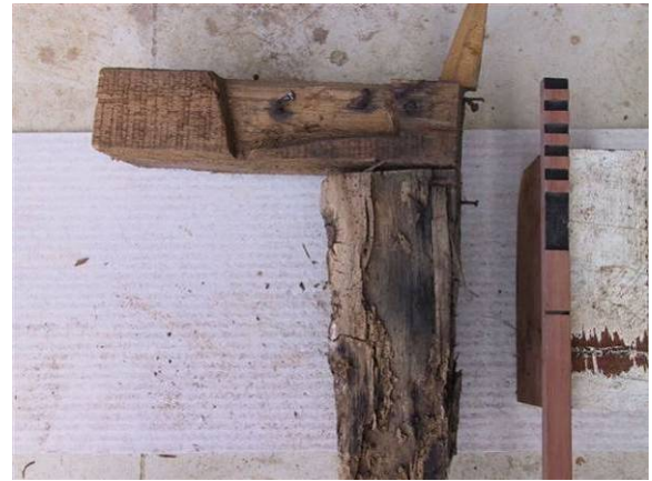
Figure 42. Bottom plate for wall and corner pile
