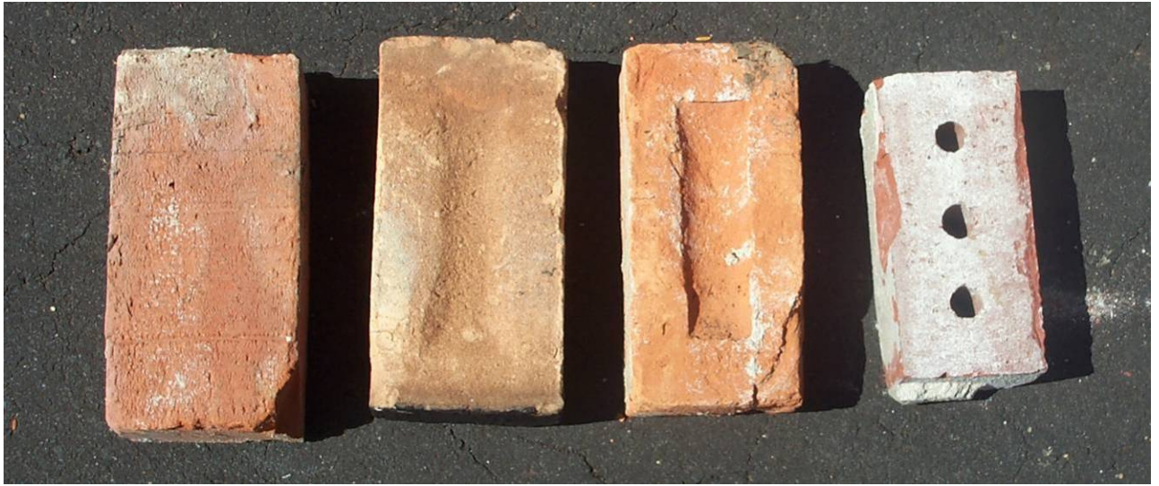
Figure 59. Range of bricks found in the house foundations
