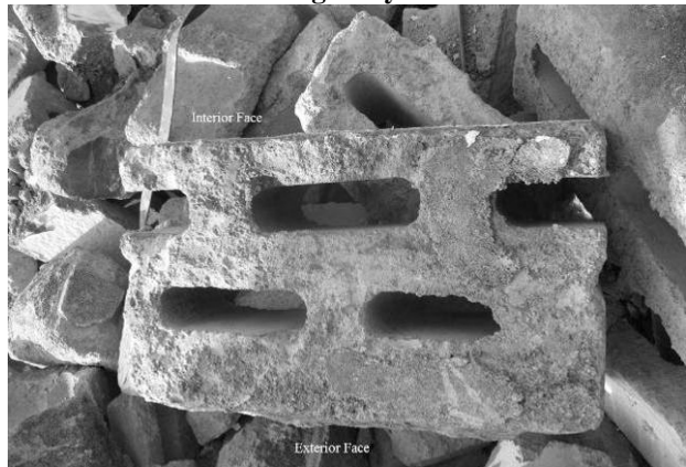
Figure 48. Example of a pre-cast air cavity cinder block
